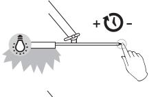
Once lamp is on > depressing push - sensor button to adjust lighting to desired settings can be done by holding push - sensor button down.
